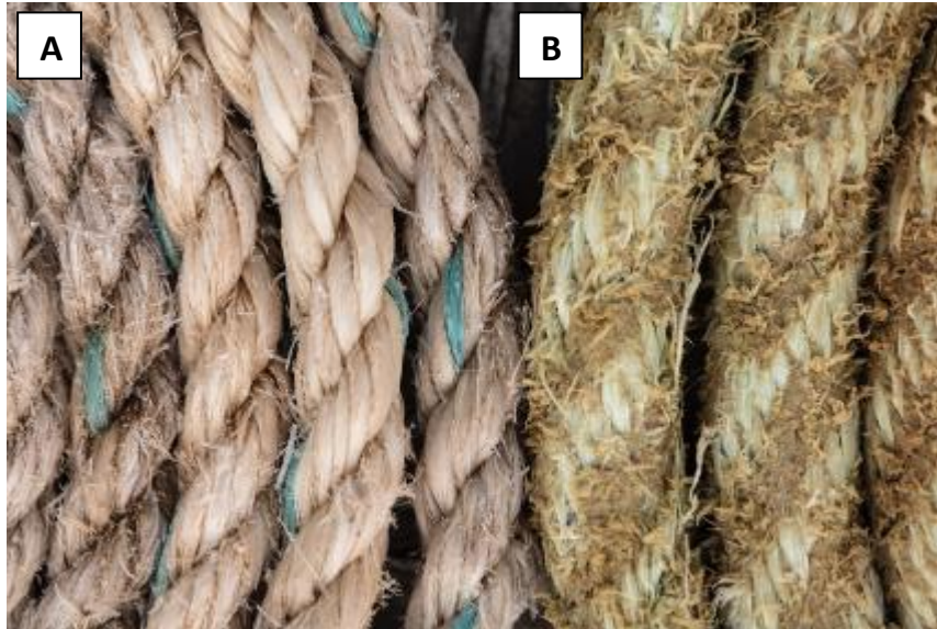
Fig. 19 (A) 10-year-old Synthetic rope (polypropylene) previously used on a recreational yacht and stored outside, and (B) 2 year-old synthetic rope (polypropylene) that has previously been used to deploy nets on a fishing vessel.
