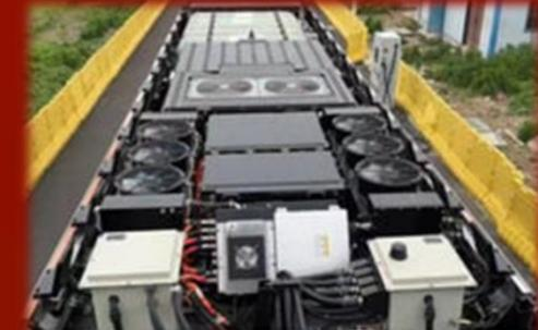
The hybrid power system on the roof
