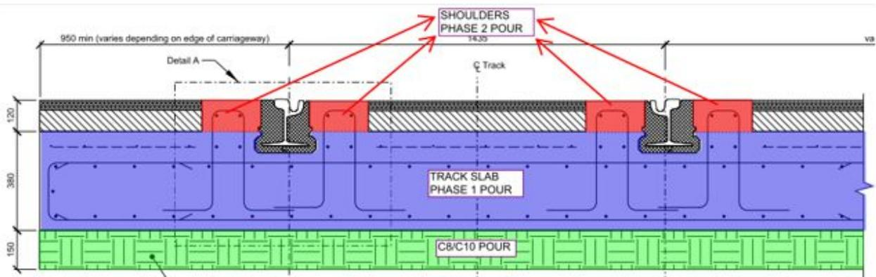
The slab is set at a depth of 500mm from finished rail level with allowance for a 150mm C8/10 blinding layer as a working platform. The choice of structural concrete for blinding is made to allow for construction traffic after an appropriate curing time and to provide sufficient strength for anchoring the props required to guarantee rail alignment.
