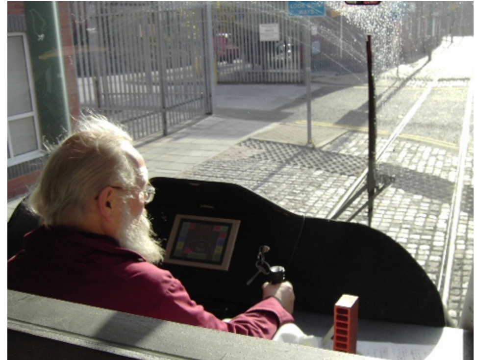
City Class Cab, with touch screen operations
