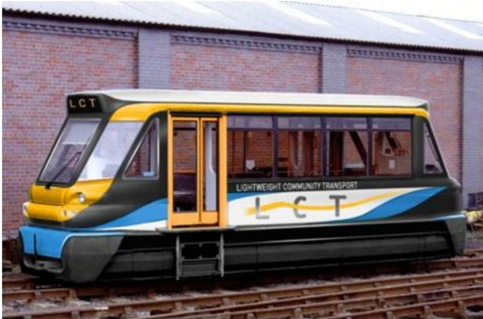
Ultra light rail does not require overhead lines; uses less energy per passenger than any other powered transport mode; is cheap to commission; and delivers a popular, user friendly service. The class 139 operated by London Midland at Stourbridge are a great example of what can be achieved: since their introduction, costs are down and passenger numbers are up. It's the most reliable and frequent service on the rail network.
