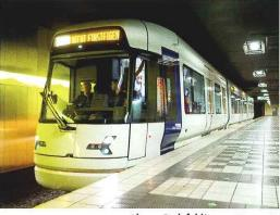
Above: Bielefeld's new Vamos HF vehicles are significant as the bulging bodies above the waistline allow 2.65m-wide car bodies to operate on infrastructure currently designed around a 2.3m-wide fleet. Heiterblick
