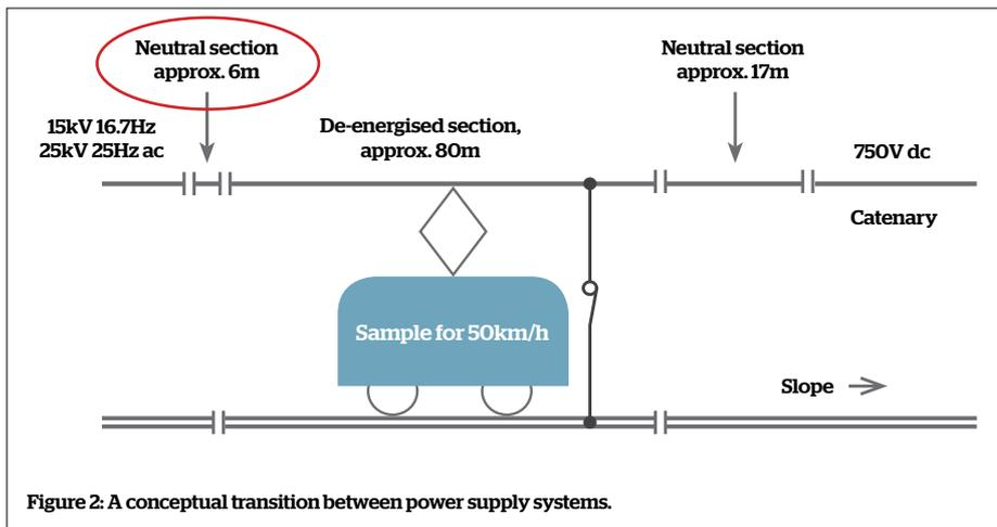
Figure 2: A conceptual transition between power supply systems.
