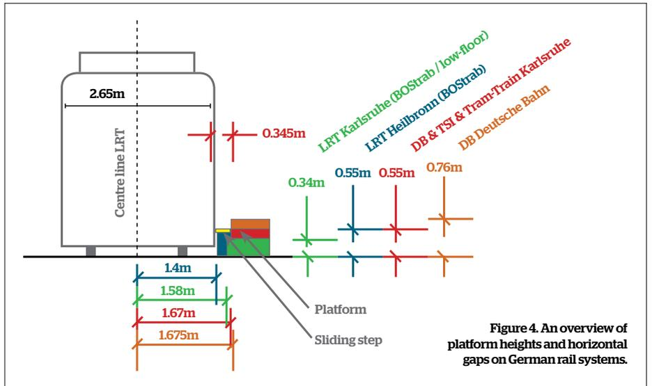
Figure 4. An overview of platform heights and horizontal gaps on German rail systems.
