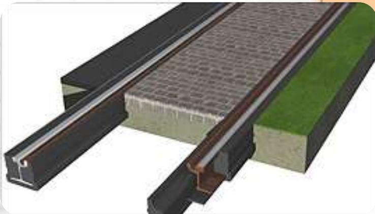
Rail encapsulated for easy replacement and maintenance
