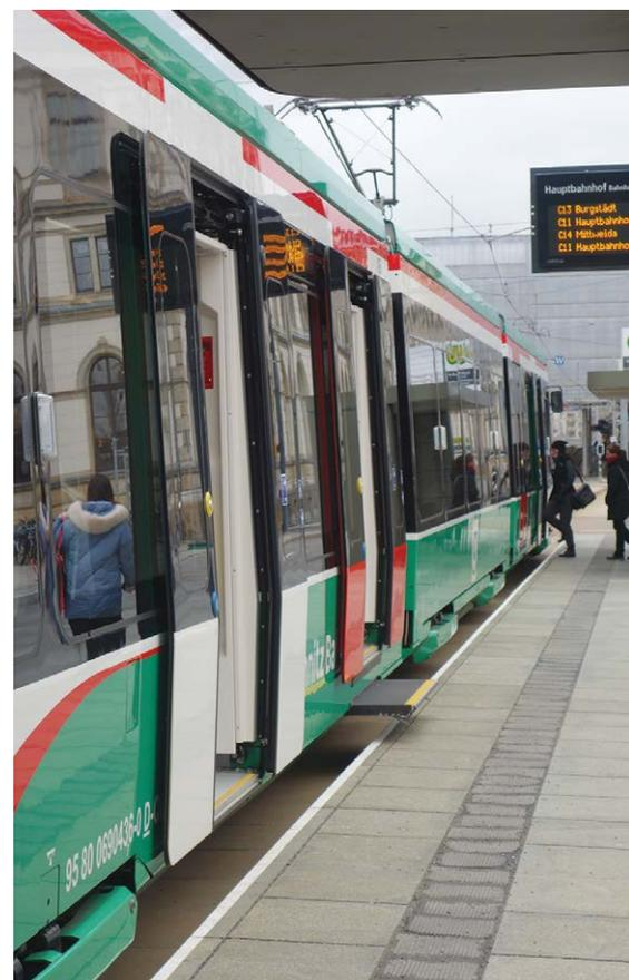
▲ Concept of low/medium-floor access points (front without and middle with moveable step) in Chemnitz. ▶
