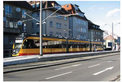
▲ A combined platform at Karlsruhe Durlach station with a height of 760mm for the Rhein-Neckar suburban railway (left) and 550mm for light rail (right).
